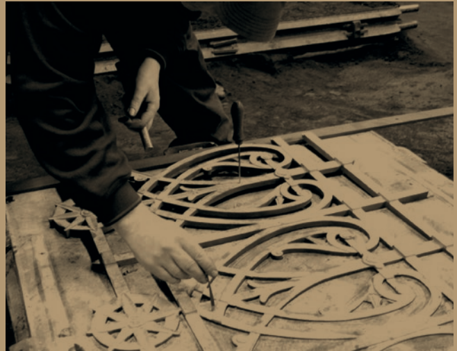
Removing the pattern from a sand mould, leaving a void into which to pour the metal
