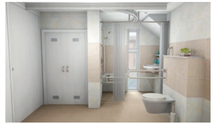
The refurbished home includes a wet room that has been designed for compliance with Part M of the Building Regulations
